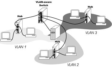
Figure 2. In this Port VLAN application, the server in the middle is logically attached to all three VLANs.
