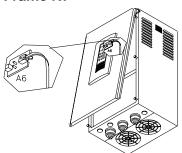
Connect the Control Panel cable to the connector X2, and replace the front cover.
