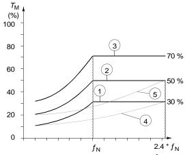
Figure 28 Underload curve types.  $T_{\rm M}$  nominal torque of the motor,  $f_{\rm N}$  nominal frequency of the motor.
