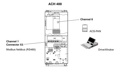
Figure 40 Standard serial communication features of ACH 400.
