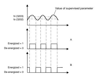
A = Parameter 1401 RELAY OUTPUT 1 (1402 RELAY OUTPUT 2) value is SUPRV1 OVER or SUPRV2 OVER
