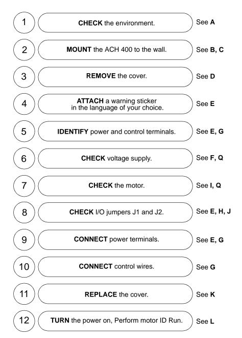
Figure 1 Step by step instructions for installing the ACH 400. The references after each step refer to one or more of the Reference Sections on the following pages in this manual.
