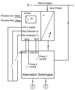
Figure 49 In this example the automatic pump alternation is in use.
