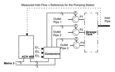
Figure 38 Regulator bypass control. The capacity of the pumping station (outlet flow) follows the measured inlet flow.
