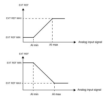
Figure 17 Setting EXT REF MINIMUM and EXT REF MAXIMUM. The range of the analog input signal is set by parameters 1301 and 1302 or parameters 1304 and 1305, depending on the analog input used.
