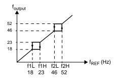
Figure 22 Example of critical frequencies setting in a fan system with bad vibrations at frequency ranges 18 Hz to 23 Hz and 46 Hz to 52 Hz.
