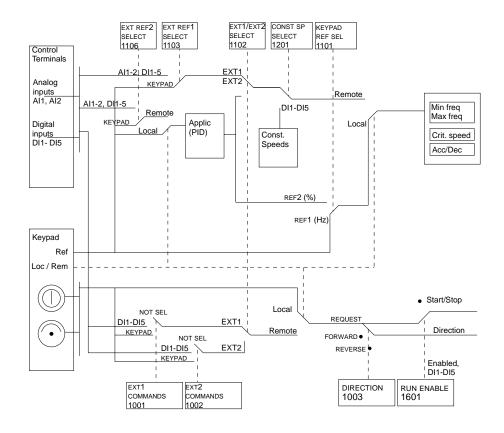
Figure 45 Selecting control location and control source.
