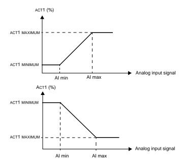
Figure 33 Actual value scaling. The range of the analog input signal is set by parameters 1301 and 1302 or parameters 1304 and 1305, depending on which analog input is used.
