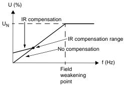
Figure 23 Operation of IR compensation
