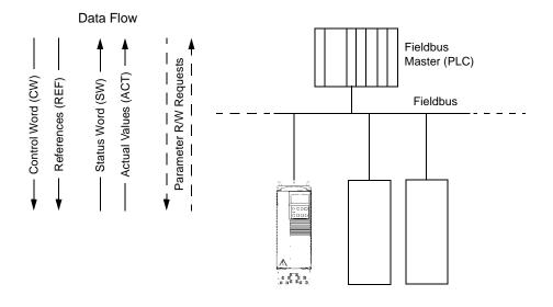
Figure 41 Structure of a fieldbus system.
