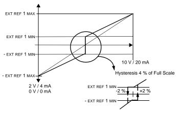
Figure 16 Joystick control. Maximum for external reference 1 is set with Parameter 1105 and minimum with Parameter 1104.
