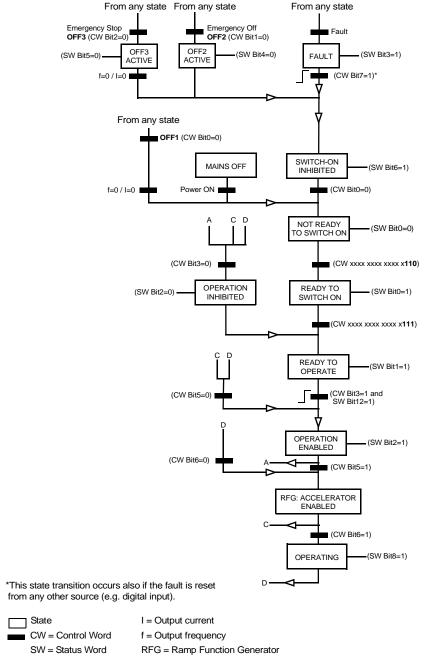
Figure 43 The state machine for evaluation of start and stop signals.
