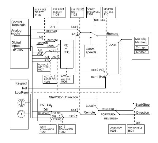
Figure 50 The control signal connections of the Pump and Fan Control (PFC) macro.
