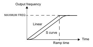
Figure 21 Definition of acceleration/deceleration ramp time.
