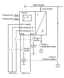
Figure 48 Operation Diagram for the Pump and Fan Control (PFC) Macro. With the default settings, automatic pump alternation is not in use.
