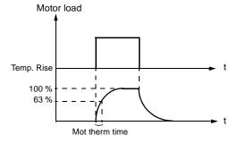
Figure 24 Motor thermal time.
