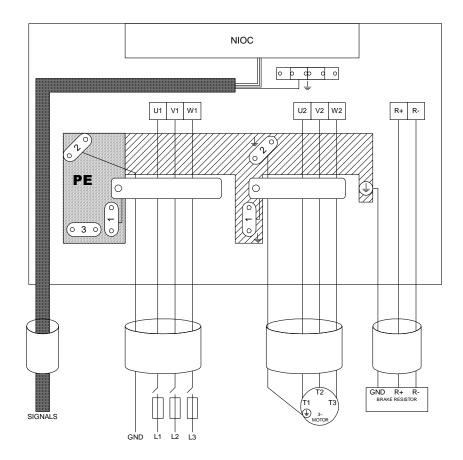
A view of the recommended wiring configuration.
