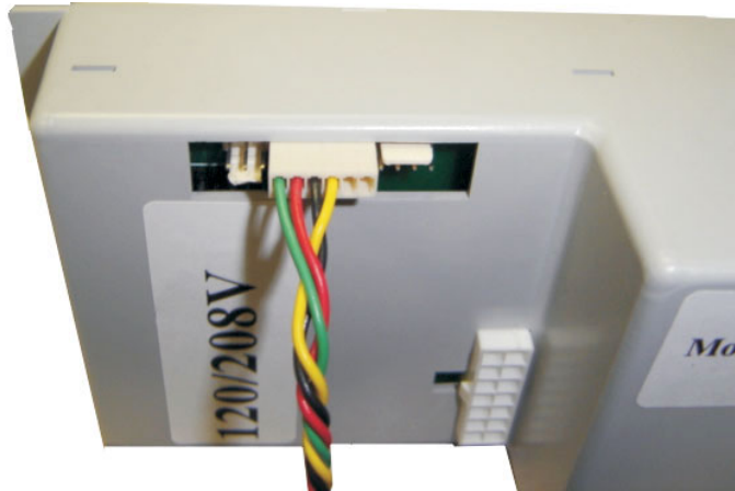
FIGURE 4–1: RS-485 Serial Connections
